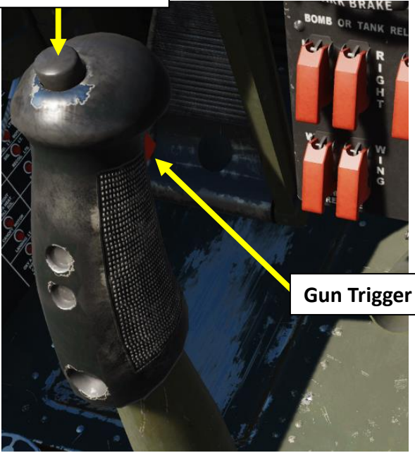
Bomb Arming Levers Turn Counter-clockwise and pull, then turn clockwise to arm. • BELLY / LEFT / RIGHT Bomb Rack
