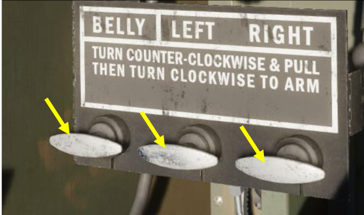
Bomb Arming Levers Turn Counter-clockwise and pull, then turn clockwise to arm. • BELLY / LEFT / RIGHT Bomb Rack
