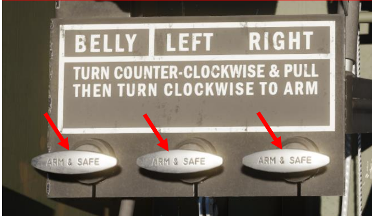
Bomb Arming Levers Turn Counter-clockwise and pull, then turn clockwise to arm. • BELLY / LEFT / RIGHT Bomb Rack
