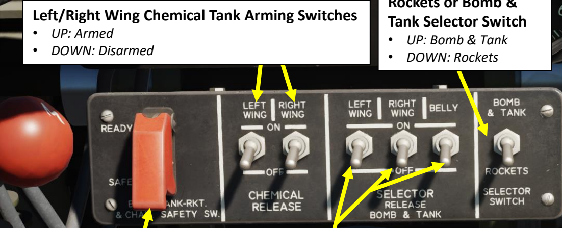
Bomb/Tank/Rocket Safety Switch (under red guard cover) • UP: Armed / Ready • DOWN: Safety is ON
